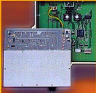
Level measurement system based on microwave radar technology. Microwave technology offers high liability and robustness at optimum price.
