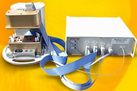
Test bench, to be integrated in a manufacturing line of electronic boards (monitoring system) for wireless application
